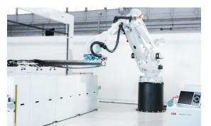
IRB 7720 is designed for high payload assembly, such as EV batteries and other heavier parts
